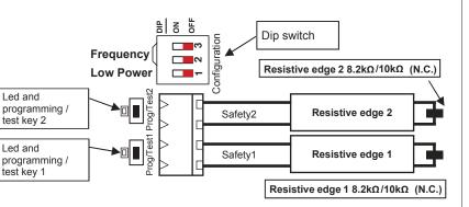
RCOO900 -  $10k\Omega$  output on both (receiver) relay 1 and relay 2.
