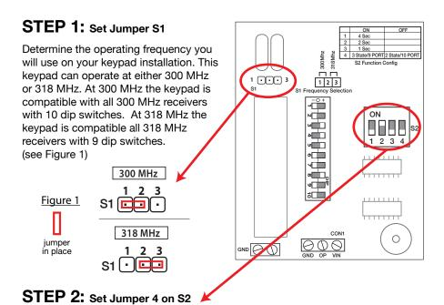
• 300 MHz (10 dip switches) - Jumper set to OFF (in the DOWN position)
