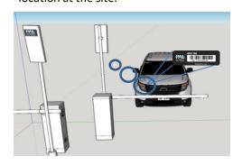
The antenna is transmitting via cone of approximately 30 degrees.
