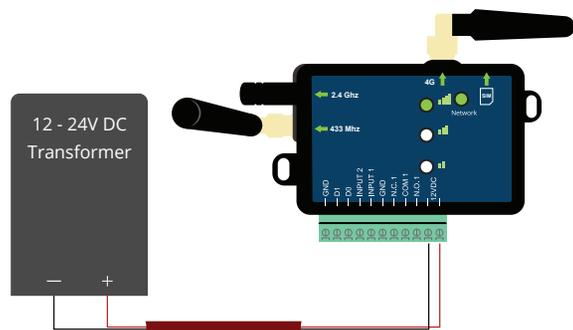
**Power** - PAL requires a 12-24V DC transformer. PAL reaches 30mA at maximum power consumption.
