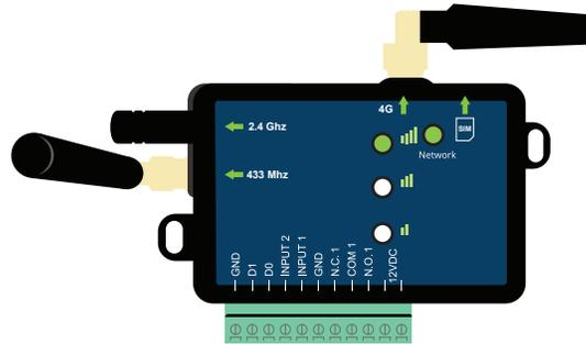
**Mounting** - When mounting the PAL be sure the RFID antenna is pointing as close to vertical as possible. For the best signal strength. The 4G antenna needs to be pointing to the right
