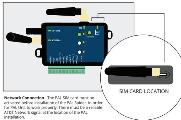
**Network Connection** - The PAL SIM card must be activated before installation of the PAL Spider. In order for PAL Unit to work properly, There must be a reliable AT&T Network signal at the location of the PAL installation.
