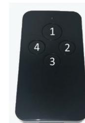
Buttons are designated 1-4 starting at the top and going clockwise around the remote.
